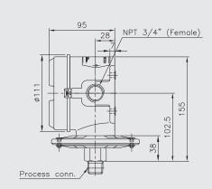
$@{-1}$  Nominal diameter Ø88 (Ø98) : 7.5  $\sim$  50 kPa (Pmax. 10 bar)
